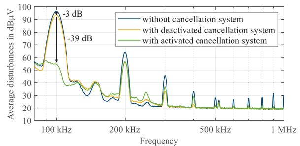
Fig. 8: Measurement results for a PFC evaluation system.
