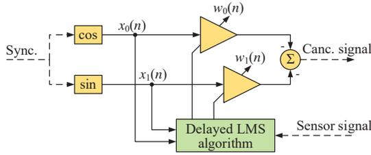
Fig. 6: Single-frequency adaptive notch filter with delayed LMS algorithm.
