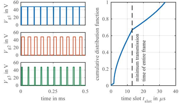
Fig. 15. Control signals of the inverter and cumulative distribution function of time slots ( $f_{\text{PWM}} = 20\text{kHz}$ )
