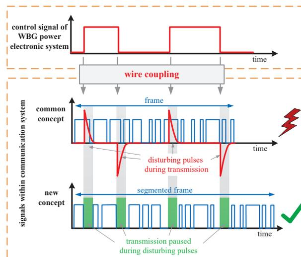
Fig. 1. Concept of adapted operation of communication based on disturbances to reduce impact on transmission
