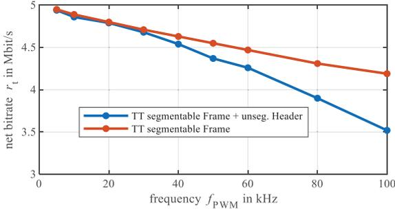
Fig. 13. Net bitrate of time-triggered CAN FD communication with segmentable frame
