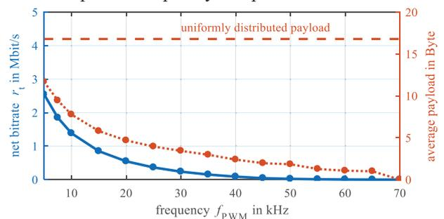
Fig. 7. Net bitrate of an event-triggered CAN FD communication and average payload of transmitted data
