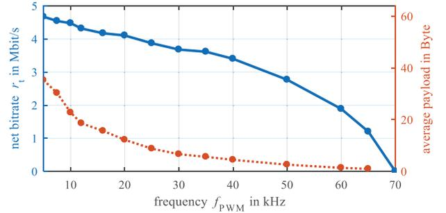
Fig. 11. Net bitrate of time-triggered CAN FD communication and average payload of transmitted data with adapted frame length
