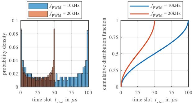
Fig. 4. Distribution of time slot duration for PWM signals with  $f_s = 50$  Hz and  $A_S/A_{\text{PWM}} = 1$  for  $f_{\text{PWM}} = 10$  kHz and  $f_{\text{PWM}} = 20$  kHz
