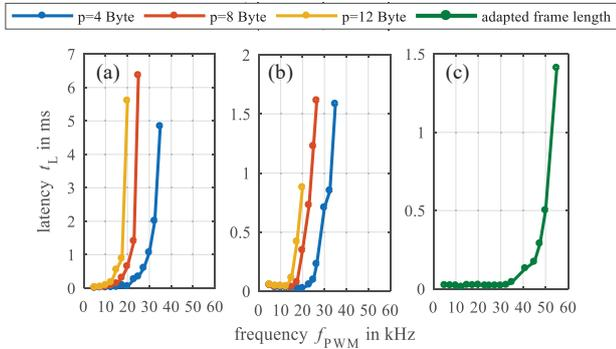
Fig. 17. Average latency of ET communication (a), TT communication with random selection of frame length (b) and TT communication with adapted frame length (c)
