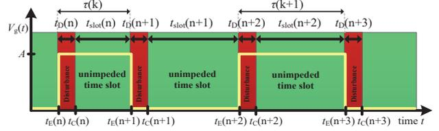
Fig. 3. General control signal (yellow), disturbance slot (red), unimpeded time slots (green) and used notation
