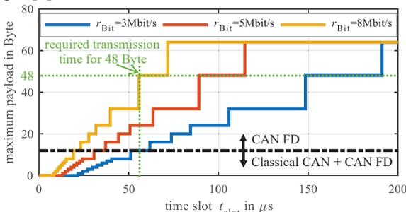
Fig. 5. Maximum transferable payload within available unimpeded slot
