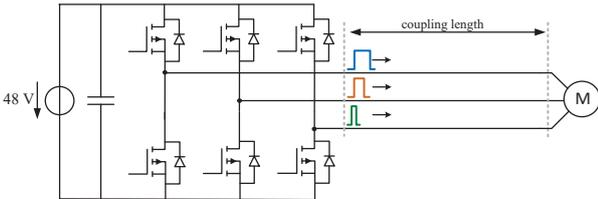
Fig. 14. DC/AC-converter as source of disturbance within a setup with cooperative operating method
