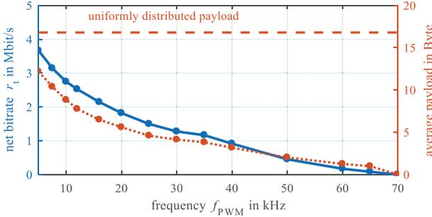
Fig. 9. Net bitrate of time-triggered CAN FD communication and average payload of transmitted data with random frame length
