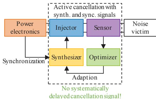
**Figure 3:** Active cancellation with synthesized and synchronized signals
