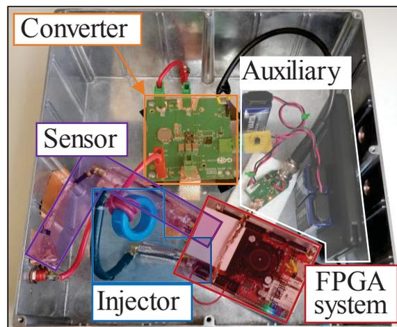
Figure 6: Photograph of the DUT
