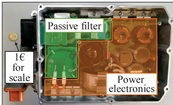
**Figure 1:** Exemplary on-board charger (3.6 kW) of KOSTAL
