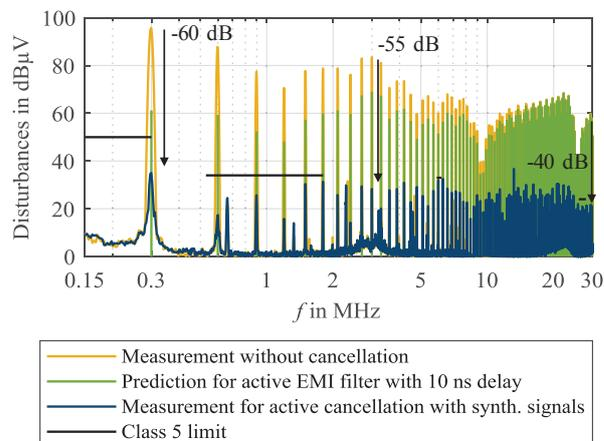
Figure 7: Measured disturbances at the artificial network
