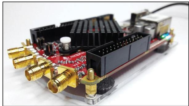
Figure 5: FPGA evaluation system with high-speed DACs and ADCs (Red Pitaya STEMLab 125-14)
