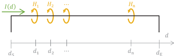
Fig. 4. Schematic presentation of the current flowing in a line and the induced magnetic field.
