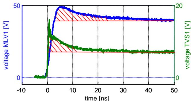
Fig. 1. Measured voltage overshoot for a MLV and TVS for a 100 V TLP pulse with 1 ns rise time
