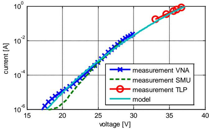
Fig. 4. IV-curve of the MLV,  $I_{MLV}(V_{MLV})$
