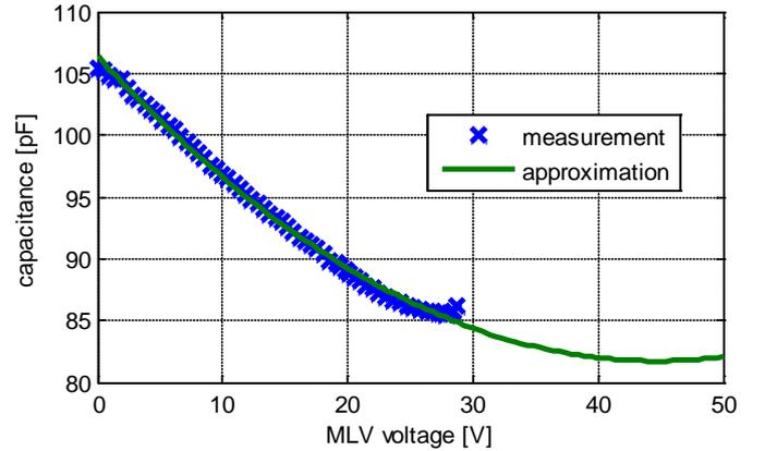
Fig. 8. Capacitance versus MLV voltage
