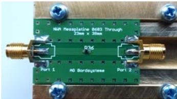
Fig. 2. Characterization PCB for impedance analysis under DC-Bias
