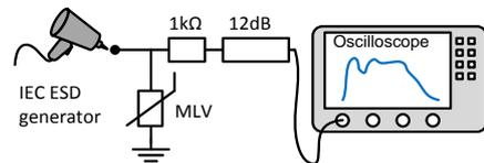
Fig. 12. Measurement and simulation setup for IEC ESD pulses
