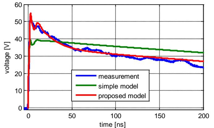
Fig. 13. Simulated and measured voltage for 1 kV IEC 61000-4-2 ESD, proposed model (red), former simple model (green)
