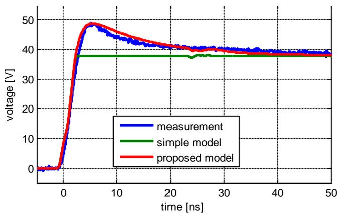
Fig. 10. Simulated and measured voltage for 100 V TLP pulse, proposed model (red), former simple model (green)
