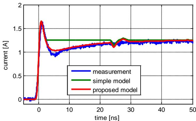
Fig. 11. Simulated and measured current for 100 V TLP pulse, proposed model (red), former simple model (green)
