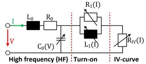
Fig. 5. MLV model including high frequency characteristic, turn-on circuitry and the static IV-curve
