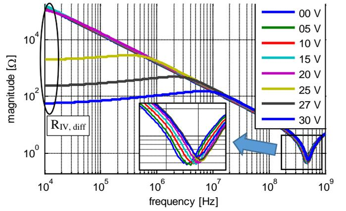
Fig. 3. Impedance  $Z_{MLV}$  of the MLV
