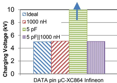
Fig. 24: Robustness on system level of μC-GPIO for different grounding
