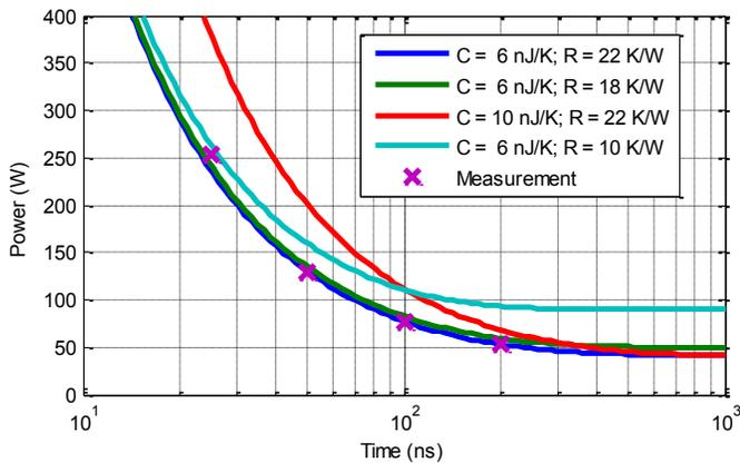
Fig. 8: Calculated and measured failure pulse power for a LIN IC (ATA6662C) for different TLP pulse width for four thermal RC network parameter sets and 900 K assumed as critical temperature
