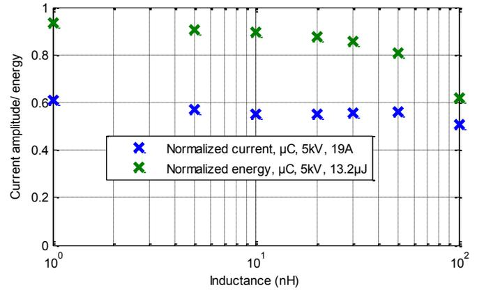
Fig. 21: Current amplitude and energy vs. inductance. Values are normalized to the initial maxima without ESD discharge
