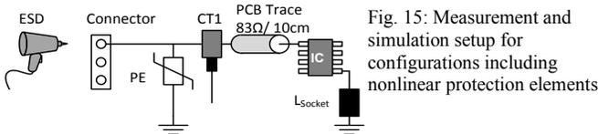
Fig. 15: Measurement and simulation setup for configurations including nonlinear protection elements
