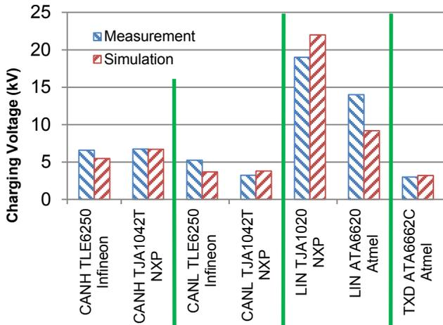
Fig. 14: Measured and simulated robustness on the system level in different configurations
