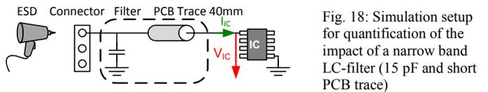
Fig. 18: Simulation setup for quantification of the impact of a narrow band LC-filter (15 pF and short PCB trace)
