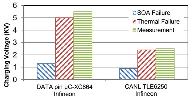
Fig. 19: Comparison of SOA and thermal failure criterion
