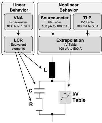
Fig. 3: Model structure and necessary measurements for model creation for nonlinear protection elements
