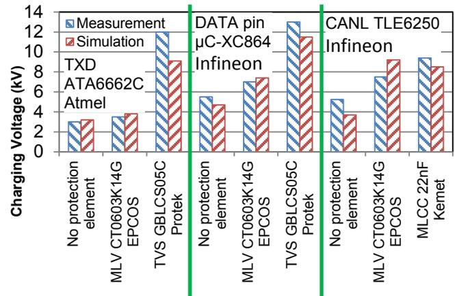
Fig. 17 Measured and simulated robustness on the system level levels in different configurations
