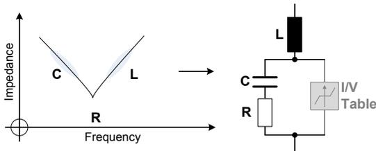
Fig. 4: Determination of equivalent models from a transfer function
