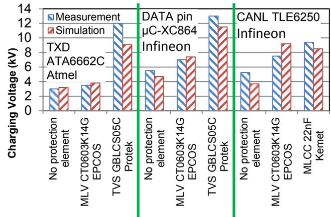
Fig. 17 Measured and simulated robustness on the system level levels in different configurations
