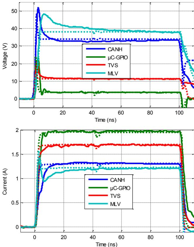
Fig. 11: Measured (solid line) and simulated (dotted line) voltage and current for TLP pulses of 100 V and 100 ns
