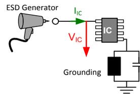
Fig. 22: Simulation setup for quantification of the impact of different grounding conditions
