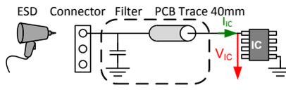
Fig. 18: Simulation setup for quantification of the impact of a narrow band LC-filter (15 pF and short PCB trace)
