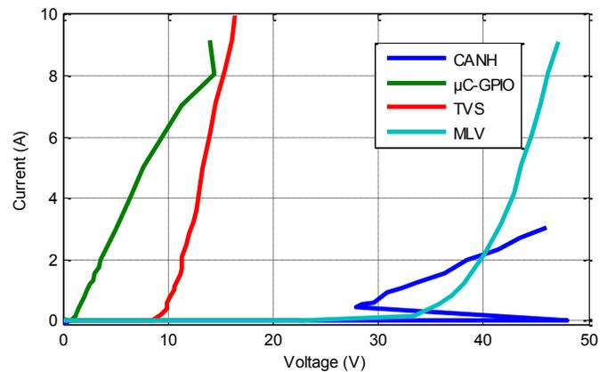
Fig. 10: Measured IV-curves for different devices, integration time 60-80 ns
