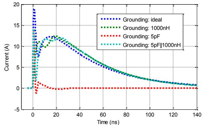
Fig. 23: Simulated current for 5 kV charging voltage on  $\mu\text{C}$ -GPIO with different grounding conditions
