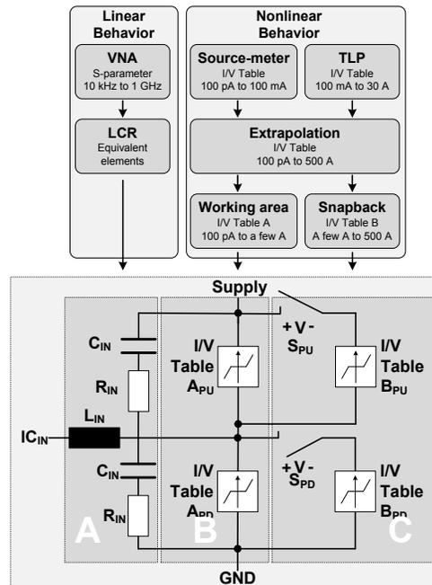
Fig. 5: Model structure and necessary measurements for model creation for IC input electric behavior
