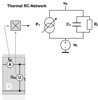
Fig. 7: General electro-thermal model
