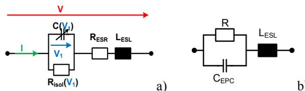
Fig. 2: Advanced equivalent circuit model of a MLCC (left), SMD resistor model (right)
