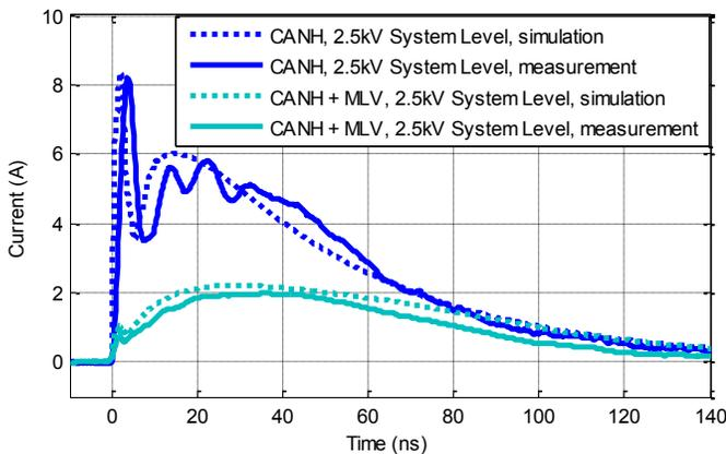
Fig. 16: Simulated and measured currents through the TJA1041T CANH-pin for 2.5 kV charging voltage with a MLV
