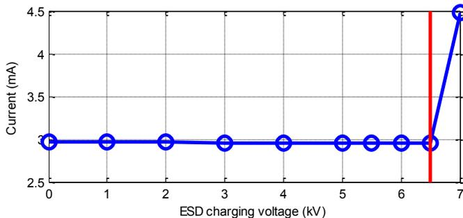
Fig. 9: Leakage current change at 40 V after ESD system level stress
