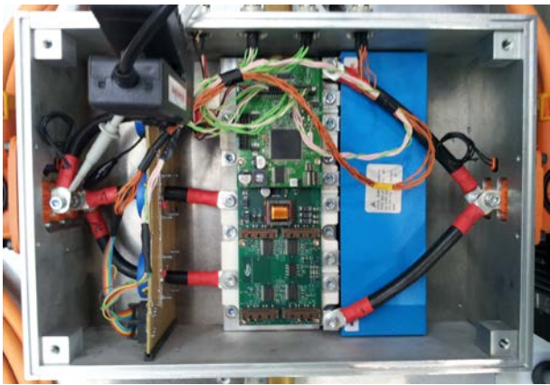
Fig. 4. INFINEON HybridPACK2 with enclosure and measurement equipment
