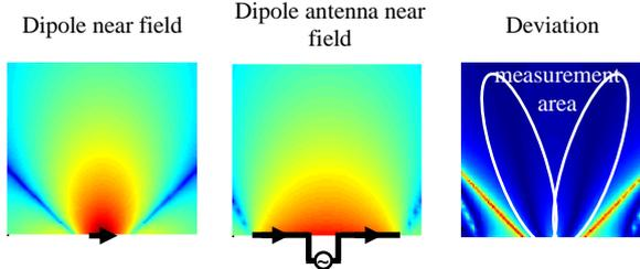
Fig. 6. Comparison of elementary dipole near field and dipole antenna near field
