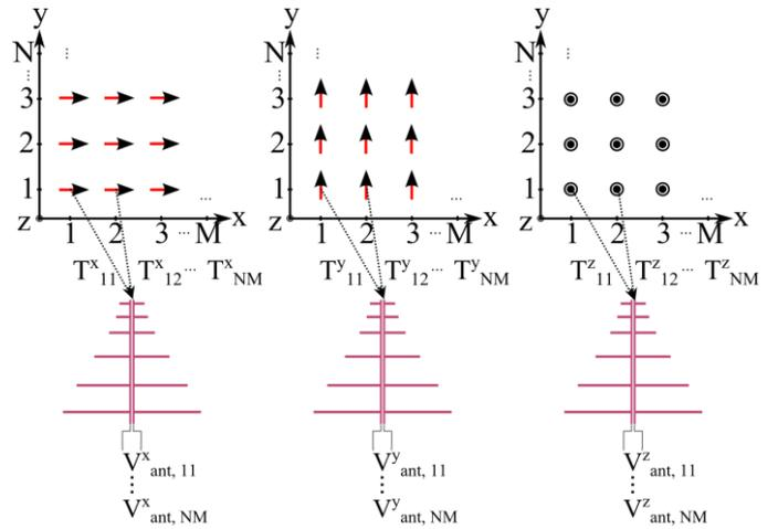
Fig. 3. Transfer function calculation of antenna voltage and impressed currents (Hertzian dipoles)
