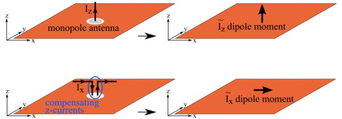
Fig. 4. Approximation of small antennas with Hertzian dipoles; monopole antenna (above) and dipole antenna (below)
