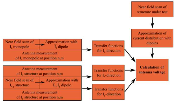
Fig. 7. Process chain of TF method
