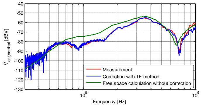
Fig. 15. Comparison of MoM simulation; TF method and real antenna measurement; vertical polarization
