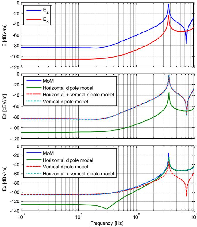
Fig. 9. Comparison of  $E_x$  and  $E_z$  components at observation point (above); Comparison of  $E_z$  fields of different dipole models (center); Comparison of  $E_x$  fields of different dipole models (below)
