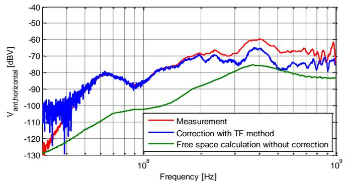
Fig. 16. Comparison of TF method and real antenna measurement; horizontal polarization
