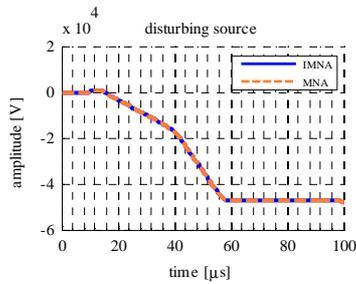
Figure 9. Shape of the disturbance source
