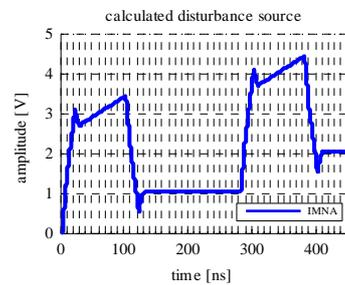
Figure 6. Shape of the disturbance source
